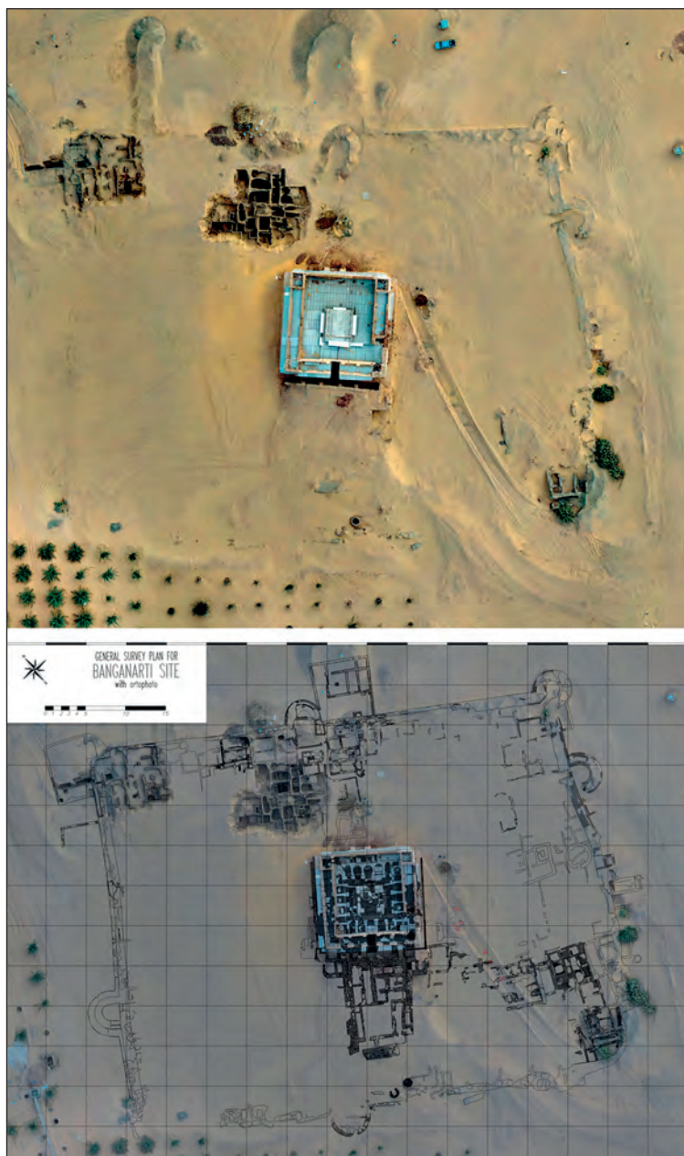
Fig. 1. Banganarti: top, airborne photography, season 2015/2016; bottom, orthophotographic image generated from the airborne photographs and geodetic measurements and overlapped with the plan of the Banganarti enclosure, February 2016 (Photo and rendering R. Łopaciuk and B. Żurawski)
